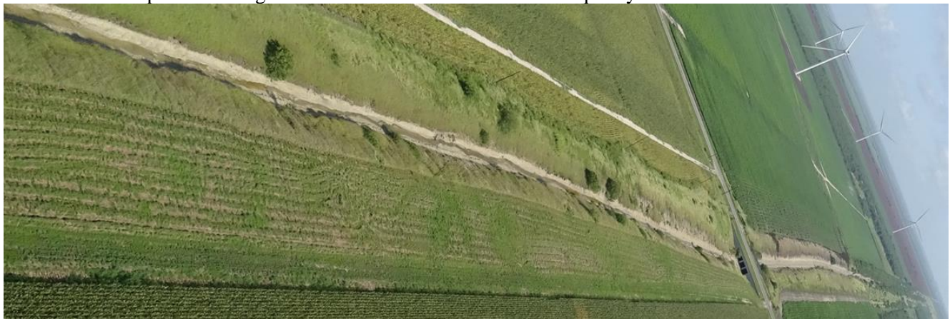
Figure 62 This image shows the Landfill Ditch stormwater drain to the Lower Reach of Petronilla Creek incised and its banks either bare or kept mowed. There appears to be a setback, perhaps an easement that restricts row crops to within 80-150 feet of the channel edge.
