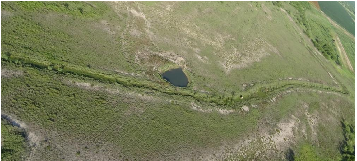
Figure 53 In this image the riparian area is hindered by farming/grazing too close. Further upstream, near the top of the image, the channel has been manipulated and straightened.
