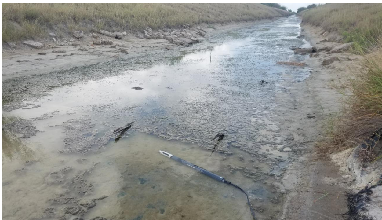
Figure 8. Hydrolab MS5 datasonde in water at Station 21598
