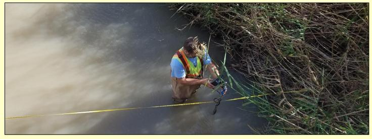
Drain using an acoustic doppler flowmeter, was 47 CFS. The water is too deep (>1.2 m) and swift for streamflow measurements using the wading rod at the Hidalgo Main Floodway.
