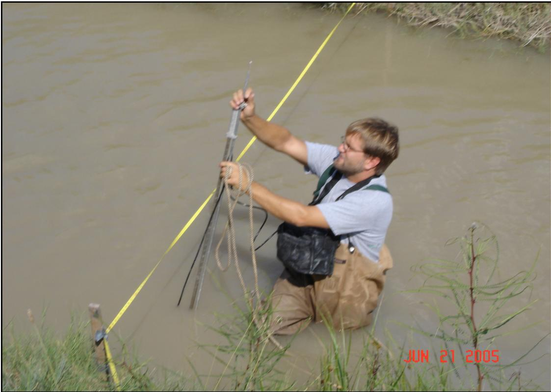
Figure 3. Photograph of Stream flow Measurement Process
